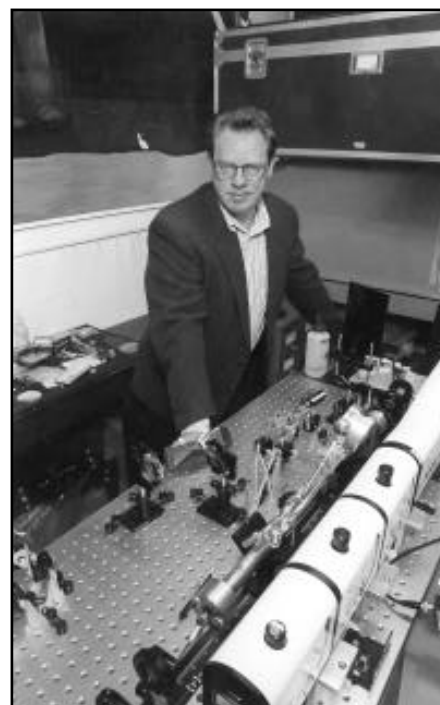
Jonathan Kenny at the portable multiwavelength laser system developed by his group for in situ detection of soil and groundwater contaminants.
