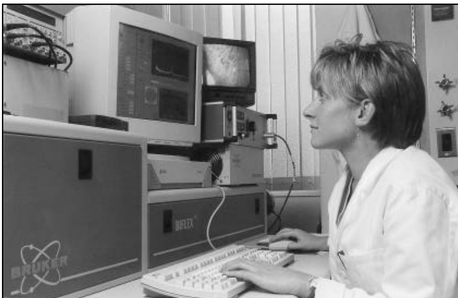
Graduate student, Colleen Bleczynski, is collecting spectra of DNA on the MALDI-TOF mass spectrometer.
